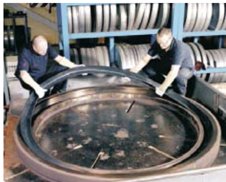
Compression moulding to 2.2m diameter.
