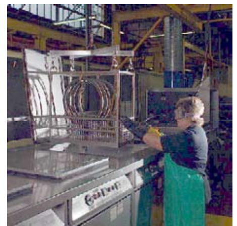
Chemical treatment of metal surfaces for top quality rubber-to-metal bonding.
