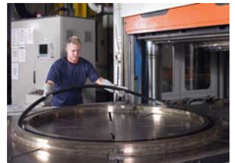
Vacuum moulding to 2m diameter.
