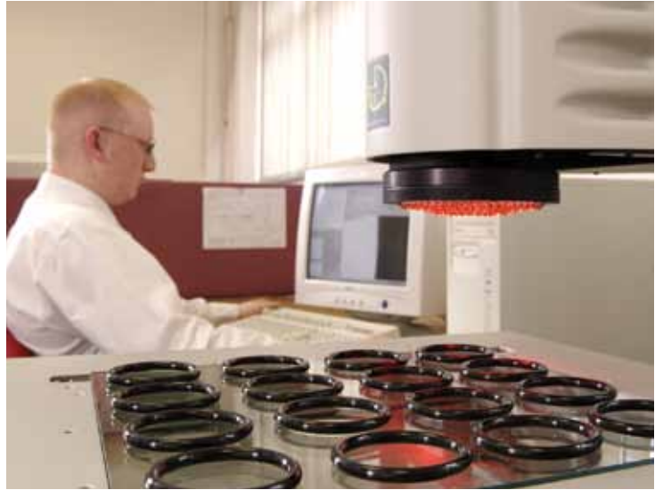
Critical inspection of elastomeric moldings with state-of-the-art optical measuring system
