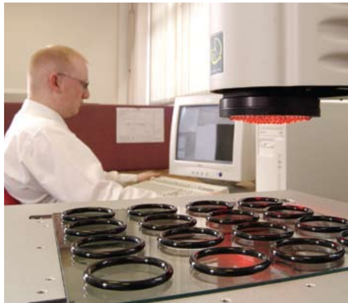
Critical inspection of elastomeric mouldings with state-of-the-art optical measuring system
