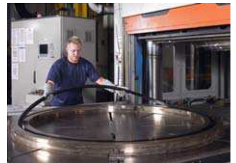
Vacuum moulding to 2m diameter.
