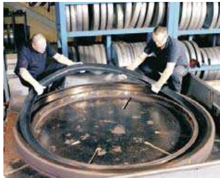
Compression moulding to 2.2m diameter.
