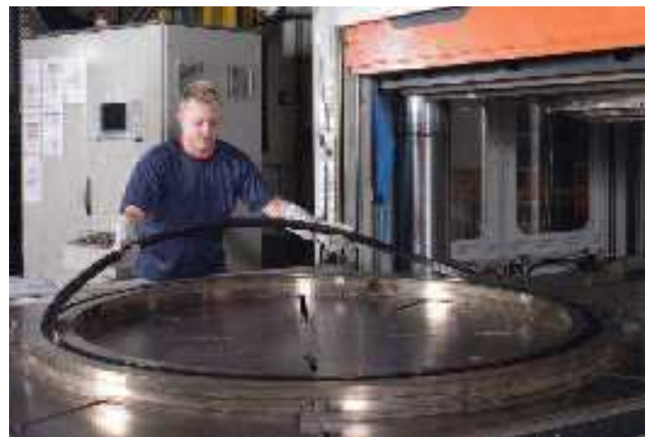
Vacuum moulding at James Walker's Cockermouth plant
