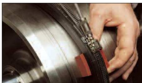
**Stage 3:** Clamp in position with steel band.
