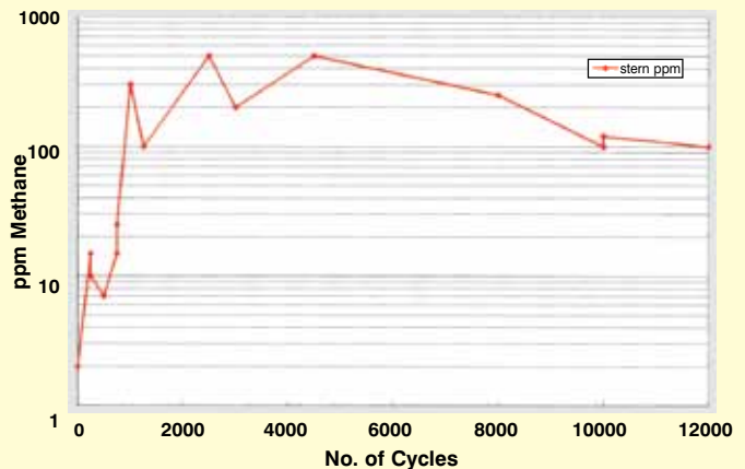
LONGEVITY TESTS: Supagraf Premier J.W. Endurance Test, - 580psi Methane
