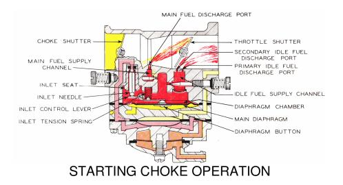
Starting an engine with the "HL" Carburetor involves the same methods that are used in a conventional float feed carburetor. However, since a diaphragm carburetor does not have the advantage of a great reservoir of fuel upon which to operate, the technique changes somewhat.
