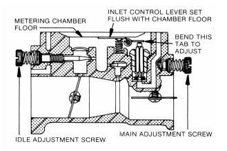
Be certain main diaphragm, gasket and cover casting are carefully fitted over the three small pins cast in rim at bottom of metering body; also the fuel pump gasket, diaphragm and fuel pump body, over similar pins at bottom rim of main diaphragm cover casting. Evenly tighten fuel pump body retaining screws to insure complete seal of casting separations at both diaphragms.
